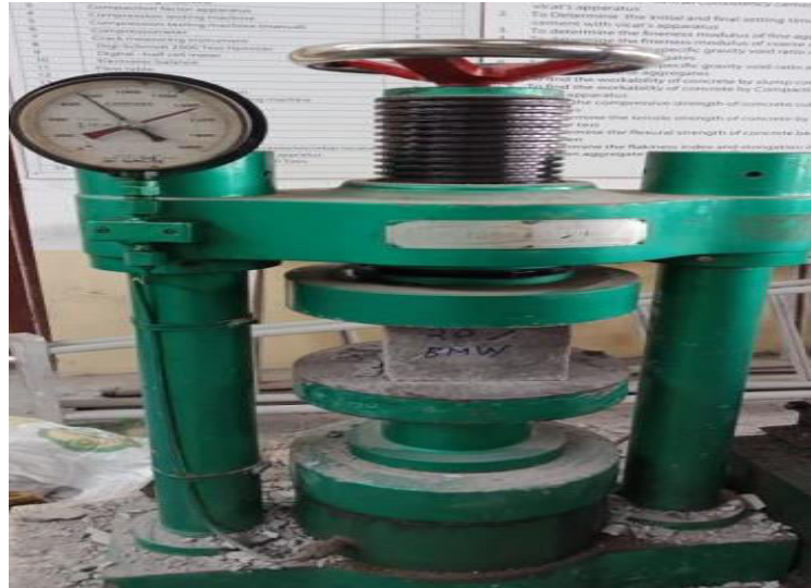
Fig. 6: Compressive strength testing of cube sample.
